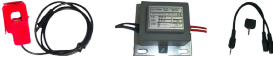
Figure 4: Sensing hardware: split-core current sensor (left), voltage transformer (center) and TRS splitter connectors (right)
