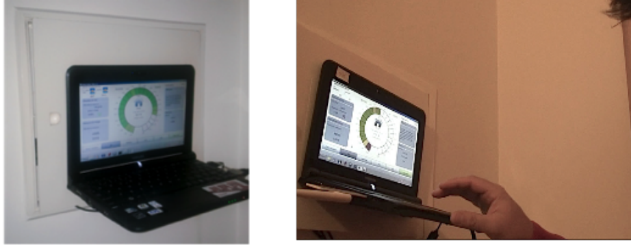
Figure 6: Energy eco-feedback is provided on-site using the netbooks' built-in LCD screen
