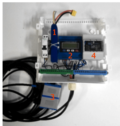
Figure 4. Box deployed with all the hardware needed for the water monitoring: (1) 3S battery, (2) TUF2000M, (3) Transducers, and (4) Raspberry Pi.
