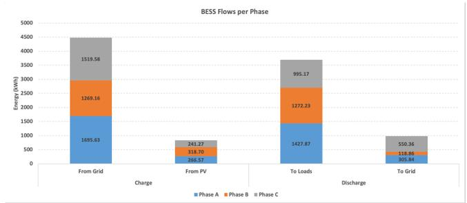
Fig. 5. Overview of BESS energy flows per phase.
